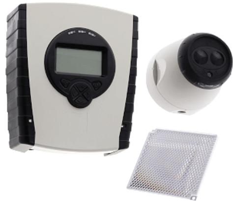
The Fireray<sup>®</sup> 5000 System is an auto-aligning, self-correcting infrared reflective beam smoke detector. Up to 2 detector heads can report to a single ground level controller. In addition, each system controller houses two pairs of fire and trouble relays, one per detector. Once the detector head is installed, using the easyfit mounting system an integral LASER can be activated. This allows the reflective prism to be located quickly and with confidence.
