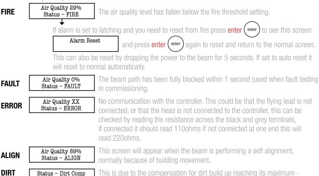
FAULT or FIRE LED may be flashing.
